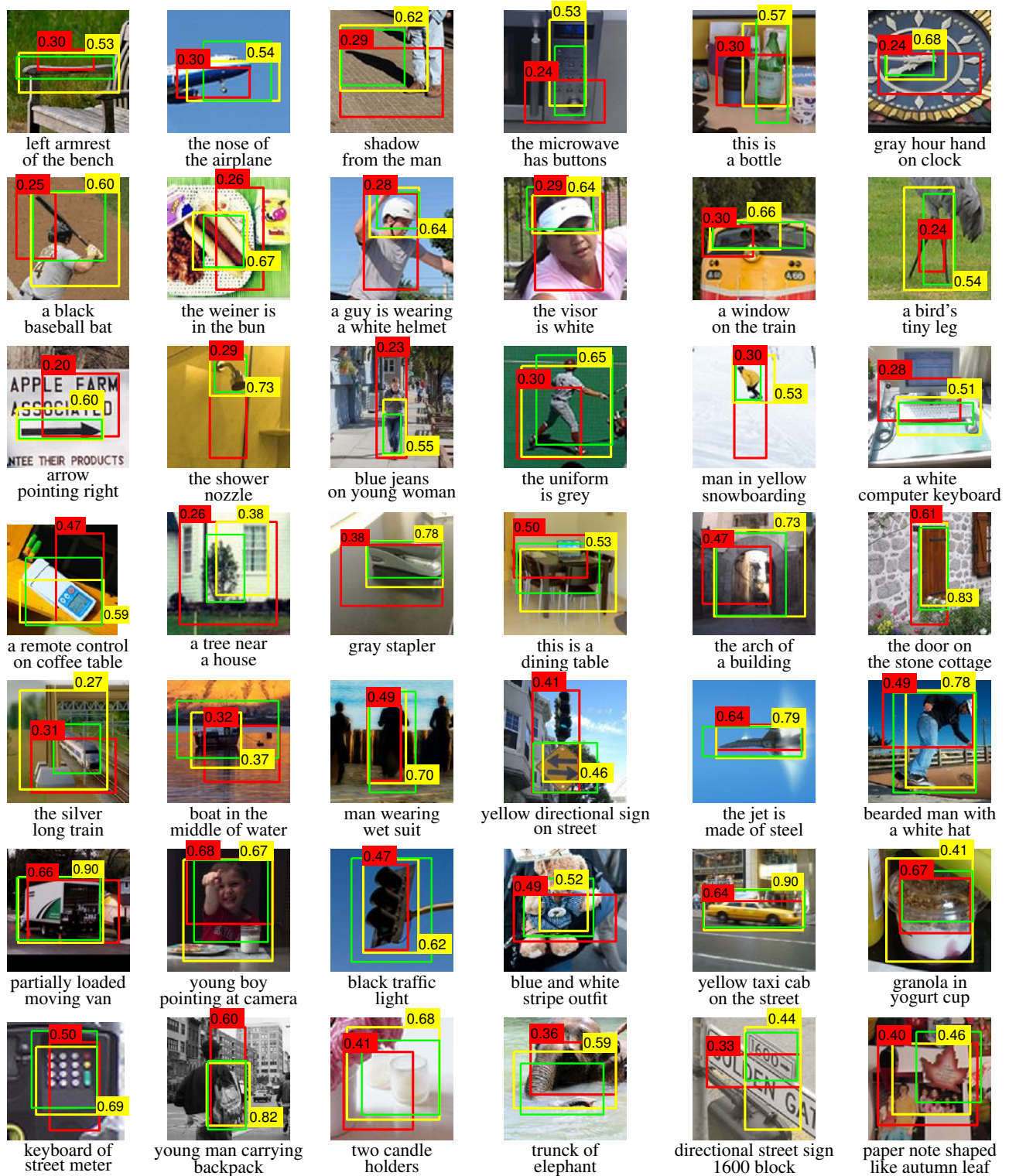
Figure 7: Qualitative comparison between DBNet and SCRC on localization task. Examples are randomly sampled. Green boxes: ground truth; Red boxes: SCRC; Yellow boxes: DBNet. The numbers are IoU with ground truth boxes.
