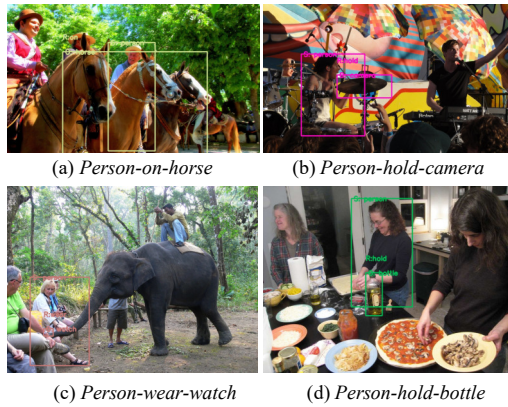
Figure 5: Visualization of a few failure cases by PST. There are four main relation detection types: (a) Inaccurate entity detection caused by crowded instances; (b) Wrong object detection; (c) Wrong association between subject and object instances; (d) Wrong predicate classification. “R” refers to predicate; “S” refers to subject; and “O” refers to object.
